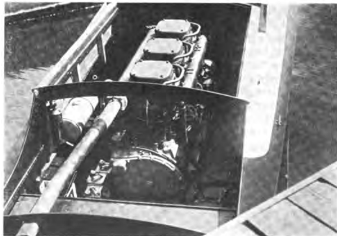
An Example of the Compact Installation Possible When Gear Drive is Used. Sterling Engine Installed in Stern of P. D. Q. VI. Speed 45 Miles per Hour
