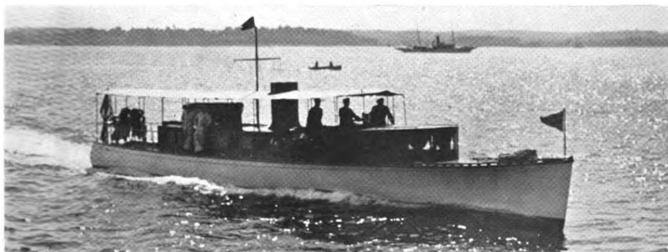
Sagitta, One of the Most Remarkable Express Yachts Ever Built. Designed Many Years Ago by Roger M. Haddock She Made 27 Miles an Hour Before that Speed had been Obtained by Anything, but an Extreme Racing Machine
