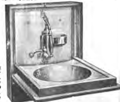
"Arco"—Plate F-691 "Arco" Folding Lavatory, N. P. copper basin and slab; N. P. composition single-acting pump; N. P. copper lining. Oak woodwork .....$34.75 Mahogany finish ..... 37.00 Height, over all, 19½"; width, 15"; depth, closed, 5½"; open, 16½"; basin 10"
