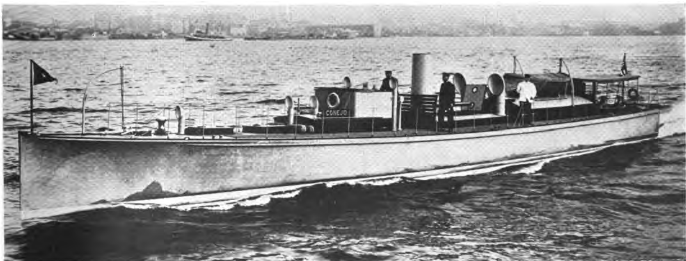
Conejo, Powered with two Sterlings, Has a Speed of Better than 30 Miles. She is Used for Fast Ferry Service
