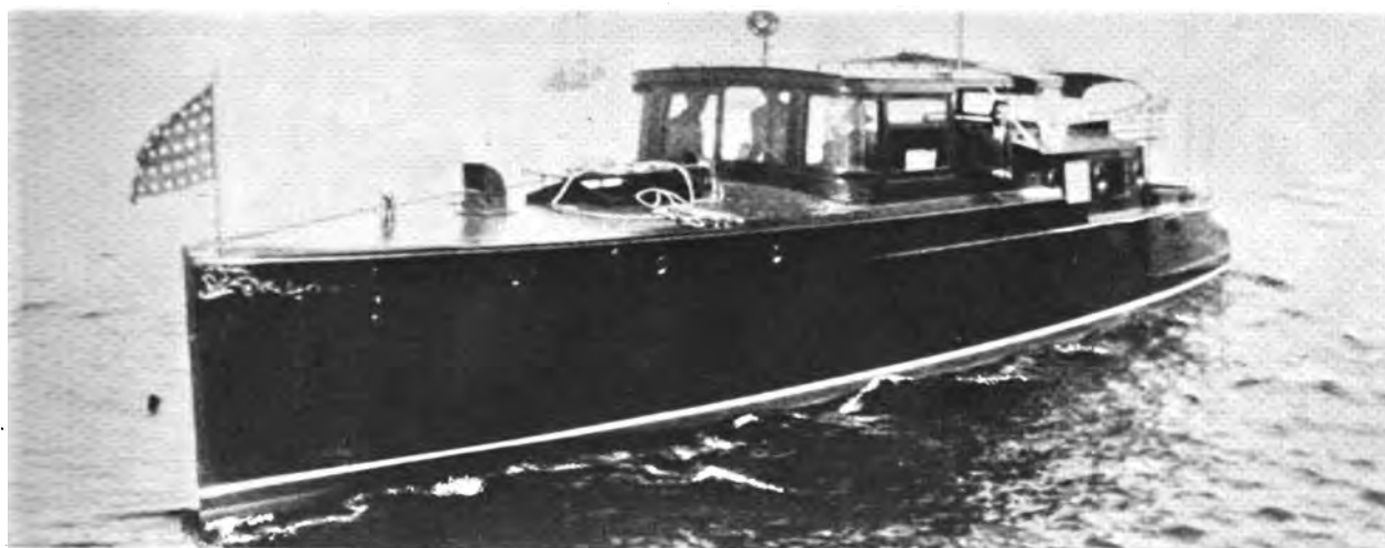
Myrno II, 50-Foot Day Cruiser, Designed and Built by Luders and Owned by Norman De Vaux, of Oakland, Cal. She is Used on Lake Tahoe, Cal., 6,000 Feet Above Sea Level. The Power Plant is a 200-H.P. Hall-Scott Marine Engine
