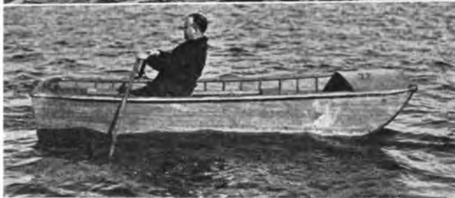
Three Views of the New Sea Sled Dinghies. Their Stability as Well as Their Adaptability with Either Oars or Outboard Engine is Well Shown. A Feature is Their Easy Towing at High Speed
