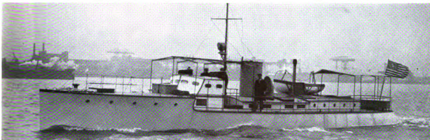
Zenith Was Designed by Bowes & Mower. Her Speed was Increased Several Miles by the Installation of a Pair of Standard Engines
