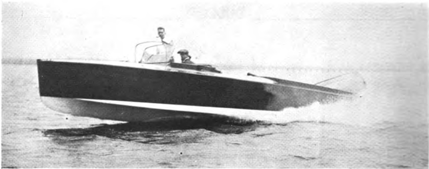
Ricochet is a Lawley-Designed and Built Runabout Powered with a 200-H.P. Hall-Scott Marine Engine. She is Owned by Horatio N. Slater, of Port Washington, Who Takes Full Enjoyment from Her 38-Mile Gait
