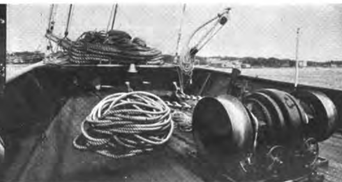
The Dash of a Runabout is Usually Arranged Like an Automobile. Large Yachts Like This One Require Electric Winches for the Handling of Ground Tackle
