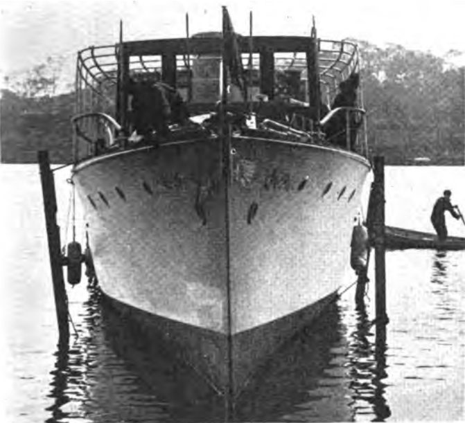
This View of Sasqua Shows the Graceful Flare and Clean Entrance that Characterizes all Luders Designs
