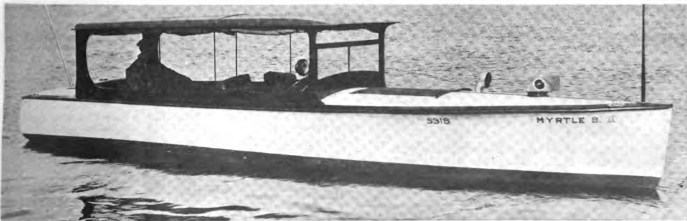
Myrtle B. II, a Stock Runabout Built by the Everett Hunter Boat Co. and Powered with a 30-40 H.P. Red Wing Engine. She Is 25 Feet 10 Inches Long, 5 Feet 6 Inches Wide and Makes 22 Miles
