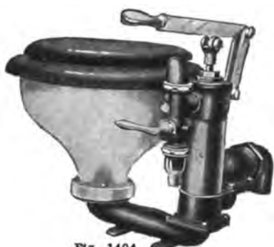
Fig. 1404 CURTISS IMPROVED MOTOR BOAT CLOSET —Dimensions 18x18 in. Height 11 in. to top of bowl. For above or below water-line. When installed above w. l. it merely requires a sea-valve on suction pipe. The inlet and outlet couplings are equipped with lead pipe cinch unions, making it possible for anyone to install. Especially adapted for small boat use, where space is limited.
