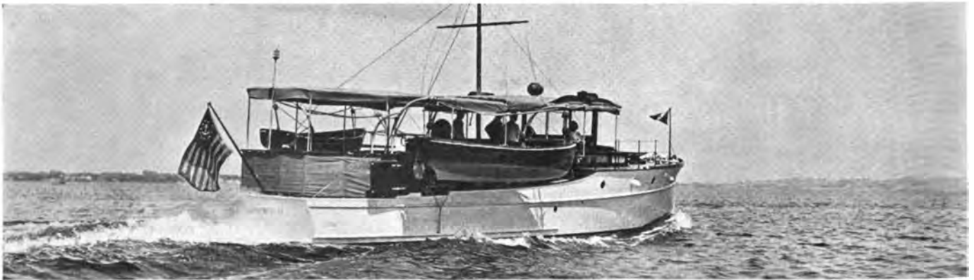
L. L. Driggs, of New York, is the Proud Owner of Grenemar II, a Sterling-Powered 50 by 11-Footer, Designed by J. H. Wells, Who is Now with the Gielow Forces. She was Built by The Matthews Boat Co. and Recently Rebuilt by Frederic S. Nock, at East Greenwich, R. I. With the 95-H.P. Sterling the Speed is 13 Miles
