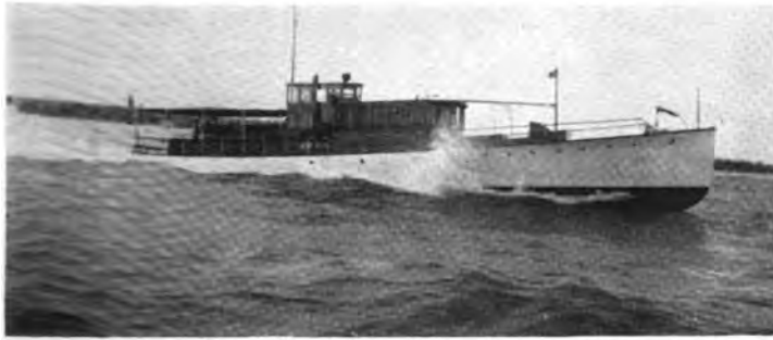
James A. Allison's Big Sea Horse, Which Failed to Start in the Havana Race. She is Powered with Two-400-H.P. Allison Engines
