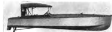
Mullins Body Corp., Salem, Ohio. 21 Ft. by 5 Ft. 6 In. by 1 Ft. 8 in. 20-H.P. Kermath. Speed 14 Miles. Price Varies with Equipment
