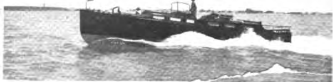
Gar Jr., II, Winner of the Ocean Races, is Powered with Two Smith-Liberty Engines, with a Total of 900-H.P. Shadow V Shown at the Right, Only Has a Total of 300-H.P., Developed by Two Speedway Engines
