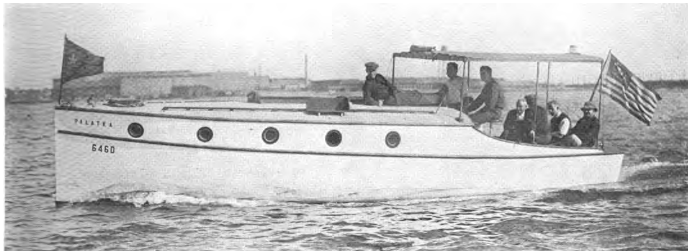
Palatka, a Raised Deck Cruiser, Owned by A. V. C. E. Hayes and Built from Rudder Plans, Which were Drawn by Bowes & Mower. Her Power Plant is a 40-H.P. Wisconsin Engine
