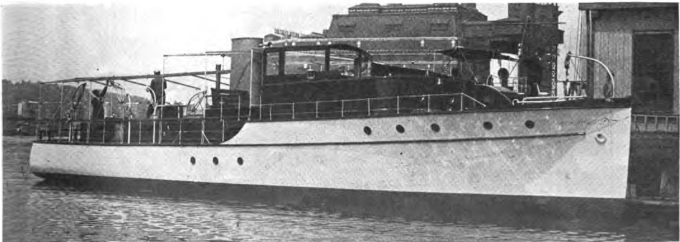
Margaret II, Latest Power Yacht to be Launched from the Consolidated Yard. She is 70 Feet by 15 Feet by 4 Feet 9 Inches Draught and is Owned by A. Roberson, of Binghamton, N. Y., Who Will Use Her on the St. Lawrence. Her Power Plant is a Pair of Speedway 150-H.P. 6 Cylinder Engines
