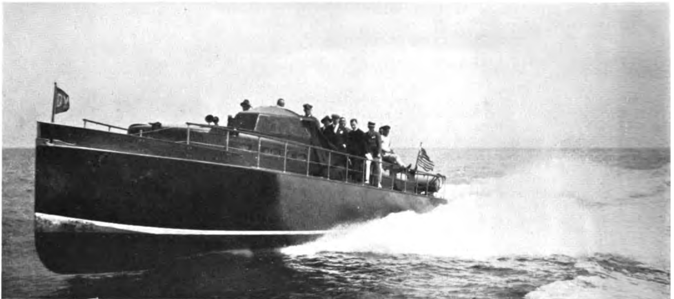
Gar Jr. II, Fastest Cabin Boat in the World. With 900-H.P. She Has an Official Speed of 41.8 Miles per Hour
