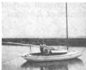
21 1/2 X 8 CABIN RUDDER CLUB DORY. BY RAISING THE SIDE ONE PLANK IT MADE A VERY SATISFACTORY CABIN CRUISING DORY.
