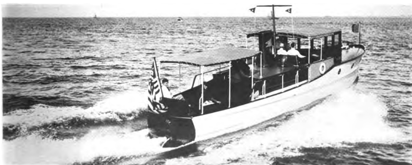
Junior, 45-Foot Cruiser, Owned by R. T. O'Dwyer, of New Orleans. She is a Hand-Designed Craft and Has a Maximum Speed of 28 Miles an Hour, with an 8-Cylinder Sterling
