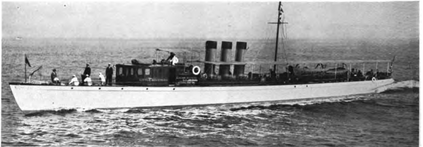
Little Sovereign Represents a More Modern Type of Fast Steamer. She was Built by Consolidated in 1909, and Had a Speed of About 35 Miles. She was Twin-Screwed and 137 Feet Long
